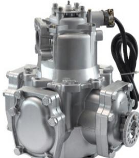
**Fm01 Flow Meter:** 4 Piston Displacement flow meter with 0.5L / revolution is specially designed for heavy duty purpose, flow range from 2 to 85 L, during this range the flow accurate can keep same result. also this meter can work without calibration for over 20 Million Liter, it is very stable.
